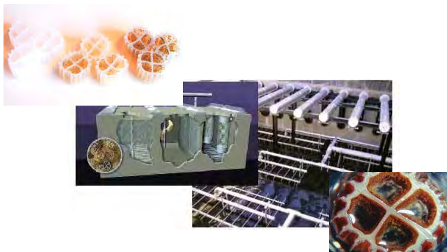
Figure 5-5 Moving Bed Biofilm Reactor
